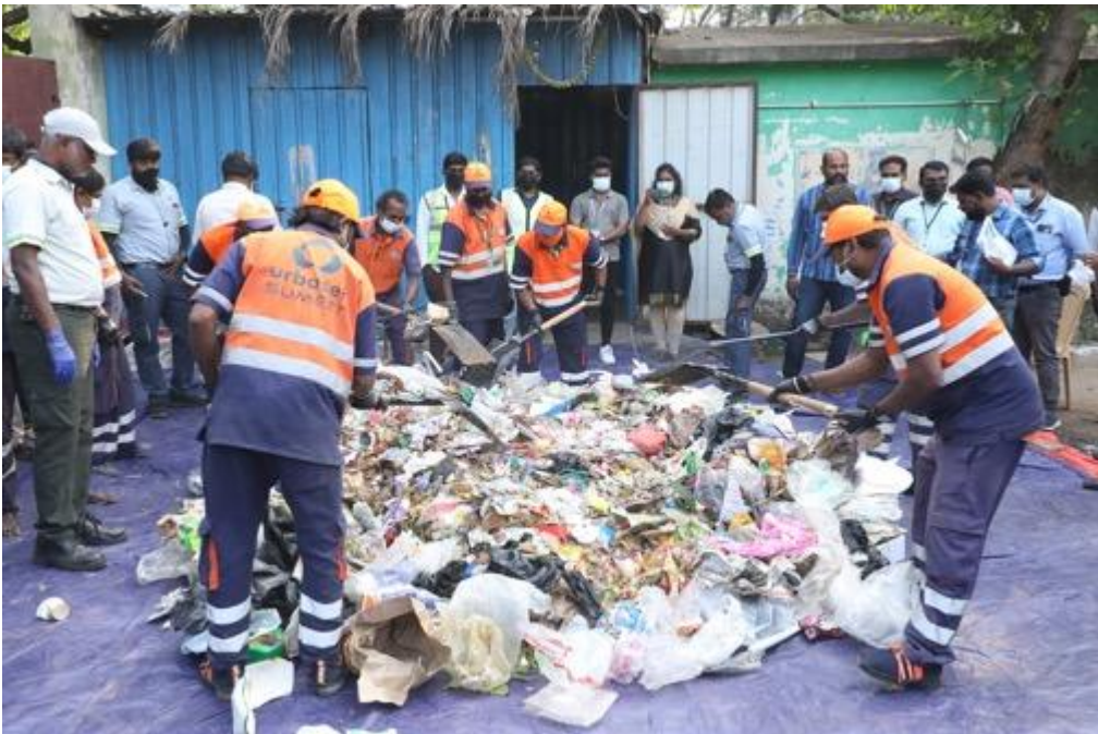
Preparation of Cone from mix waste
