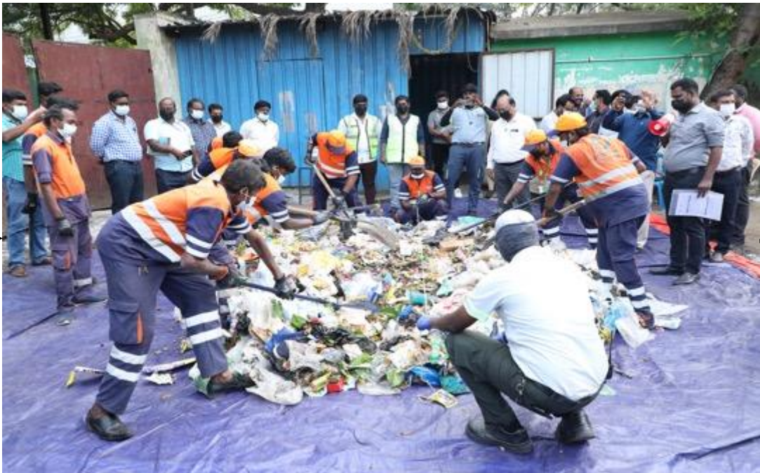
Flattening & partitioning of the cone into two parts
