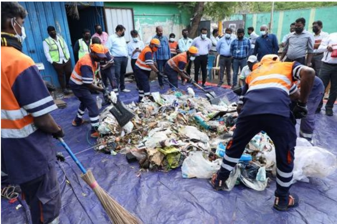
Mix the two selected quarters into one and repeat the process again
